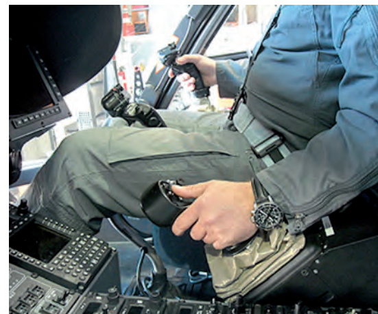
Figure 4: Active cyclic and collective stick in the cockpit of the FHS
